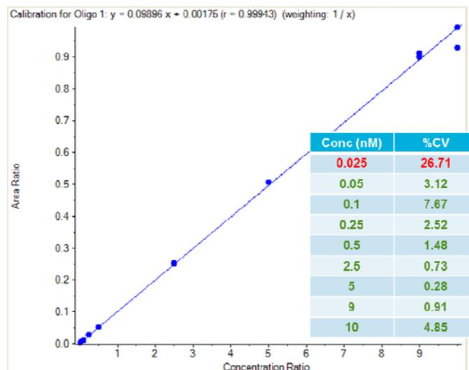
Figure 7: Standard Concentration Curve for Oligonucleotide 1 in Matrix using MRM<sup>HR</sup> Workflow. Concentration curve for Oligonucleotide 1 in plasma, using Oligonucleotide 2 as an internal standard. Using MRM<sup>HR</sup>, excellent linearity was observed, with a lower limit of quantitation of 0.05 nM.
