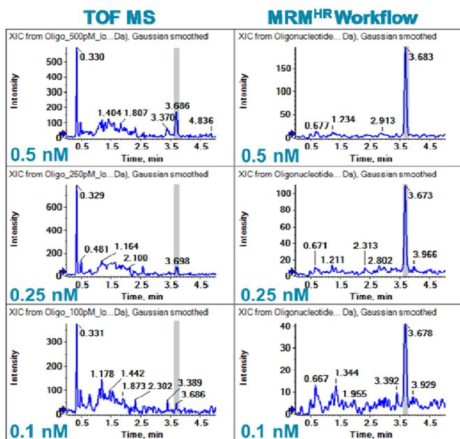
Figure 6: Selectivity of MRM<sup>HR</sup> Workflow in Complex Matrices Allows Better LLOQs to be Obtained. In the case of Oligonucleotide 1, background interferences in full scan TOF MS result in higher limits of detection and quantitation (0.5 nM), while the selectivity of the MRM<sup>HR</sup> workflow allows quantitation of concentrations less than 0.1 nM.
