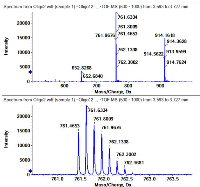
Figure 3: TOFMS Analysis of Intact Oligonucleotide 1 acquired on the TripleTOF<sup>®</sup> 5600 system (top). Isotope resolution of higher charge states is achieved with a resolution of 30,000-40,000, as illustrated by zooming in on the 6<sup>+</sup> charge state (bottom). This resolution is achieved at TOF MS scan speeds of 10 MS spectra per second.
