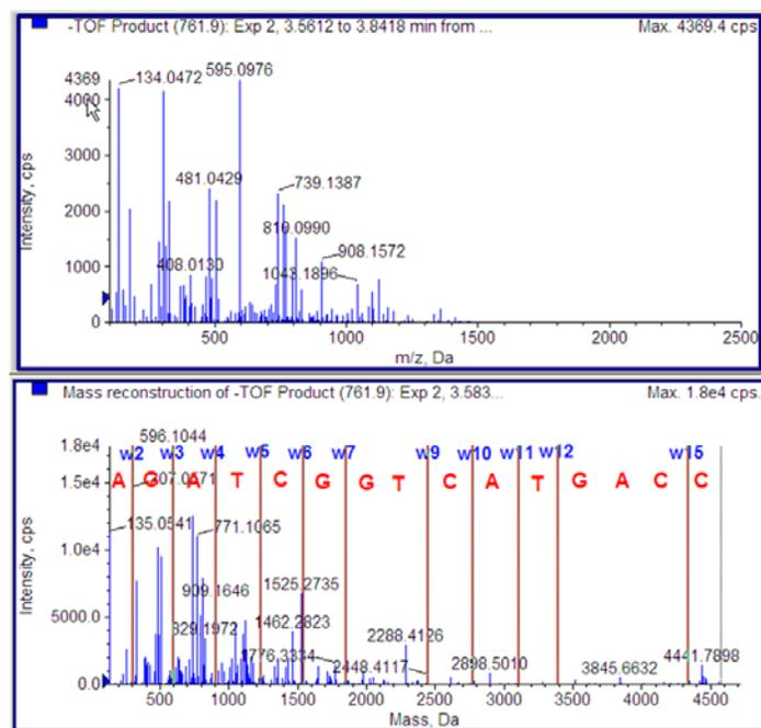
Figure 4: High Quality MS/MS of Oligonucleotide 1 for Characterization and Quantitation Method Development. (top) The full scan MS/MS approach of MRM<sup>HR</sup> workflow enables full qualitative analysis of any targeted analyte. Full sequencing of Oligonucleotide 1 was achieved on the mass reconstructed MS/MS spectrum (bottom) for fragment ion selection.
