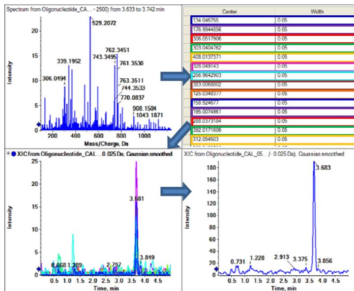
Figure 2: Principle of MRM<sup>HR</sup> Workflow Quantitation. Looped full scan MS/MS spectra are acquired for each precursor. Selected fragments are then extracted post-acquisition using narrow extraction widths (in this case 50 mDa) to produce high resolution XICs. These XICs can be used individually or summed, depending on which provides the best selectivity and sensitivity for quantitation.
